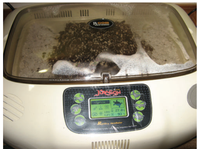
An incubator that can provide two different temperature setpoints per day gives added flexibility.
